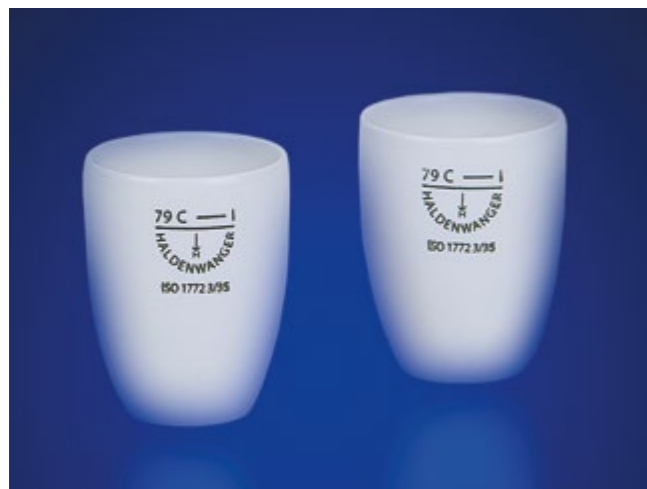
Haldenwanger crucibles shown before (left) and after (right) anneal testing. The result confirms the thermal stability of the glazing, even after multiple testing cycles.
